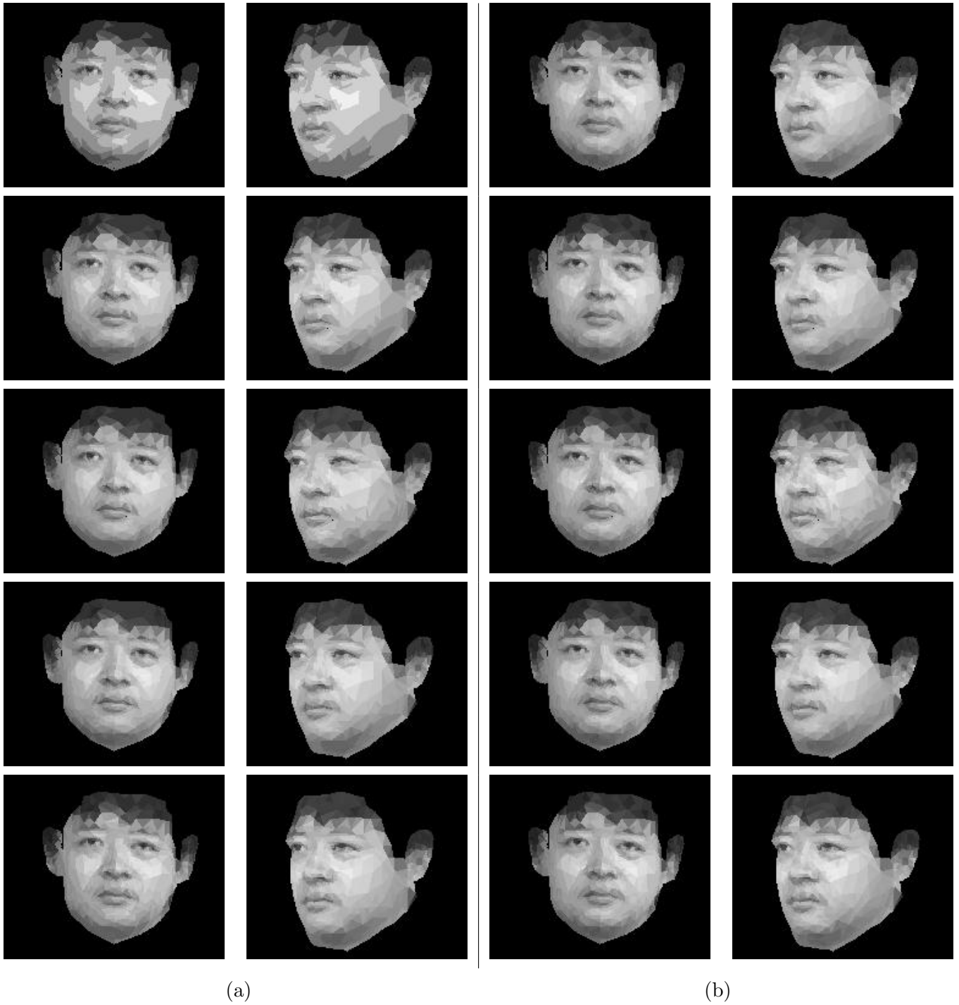
Figure 7: Coding using the TCI technique for feature extraction. (a) Separate coding of the two views using Scheme 1 with bit rate \approx 41 kbps and PSNR \approx 23.9 dB. (b) Distributed coding using Scheme 2 and PD-type side information with the same bit rate PSNR \approx 25.5 dB.
