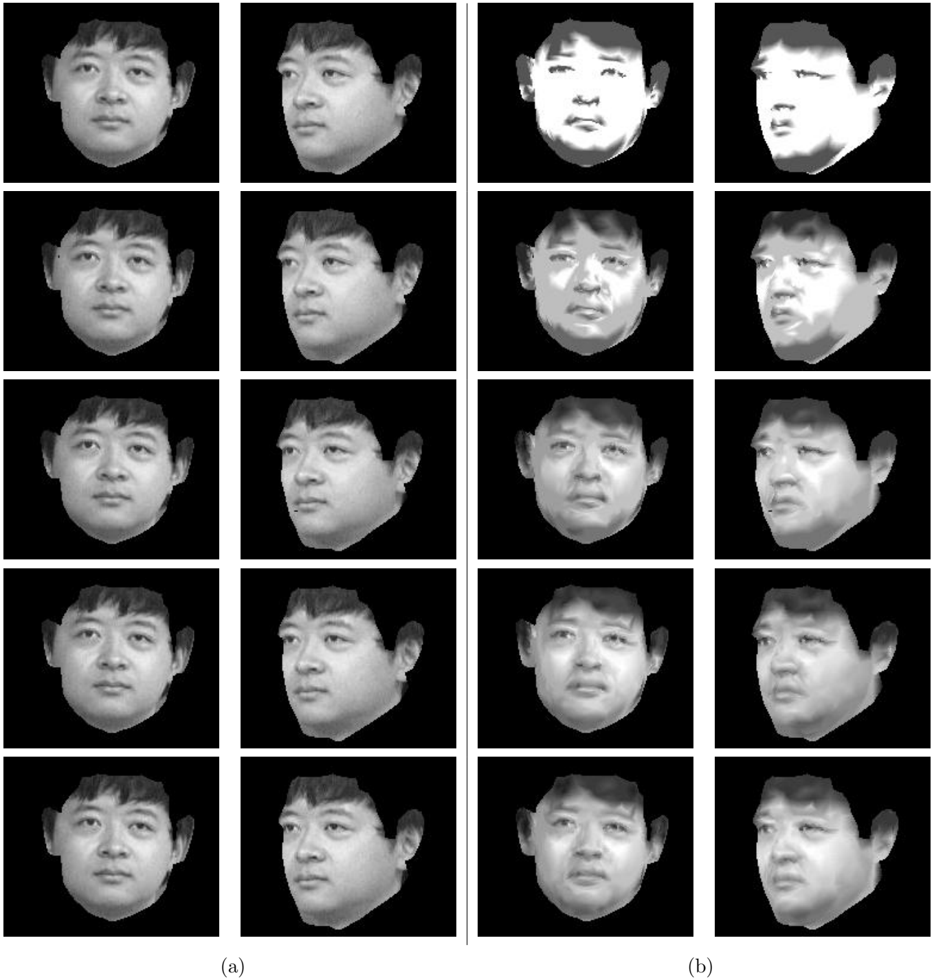
Figure 4: (a) Five consecutive frames from the original sequence. (b) Separate coding of the two views using the PSI technique and Scheme 1. The bit rate is \approx 20 kbps and the PSNR is \approx 16.5 dB.
